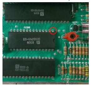
2600 Rev 16+: Lift pin 4 of 555 chip & connect to reset. Add 1K resistor as shown.
