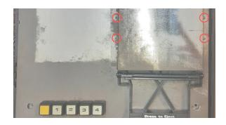
The keys should pop right off, which will be necessary for lifting the main shielding.
