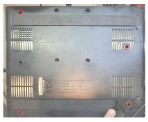
Remove the 4 screws, including one underneath the rubber foot.
