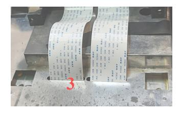
Finally, for step 3, insert through the holes in the main shielding, and then into the motherboard. If you have trouble with reach, make sure the cartridge bay is flush with the main shielding, and optionally insert a cartridge so that the springy part will give you more clearance.
